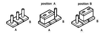
To move a jumper from one position to the other, use needle-nose pliers or tweezers to pull it off its pins and gently move it to the desired position.
